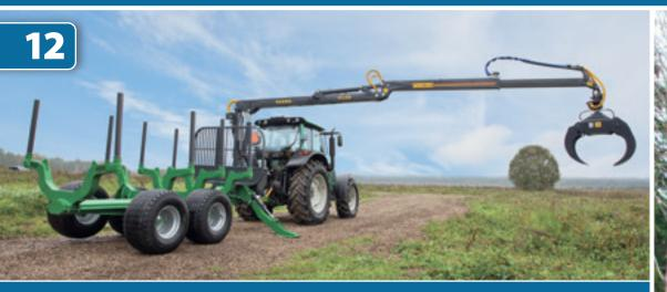
The FARMA C 7.0 is one of the market's most well-thought out and best value-for-money cranes. The crane has a reach of 7.0 m with single extension. The lifting power and movement geometry are exceptional. The attractive design, together with the choice of material, give a low dead weight.
